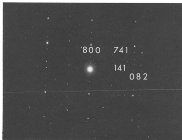
Figure 8 ED diagram of zone \langle 014 \rangle djurleite film.
