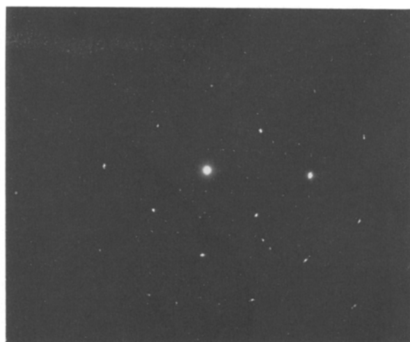
Figure 7 ED pattern of a mixture of djurleite variants, \langle 102 \rangle and \langle 232 \rangle zones.
